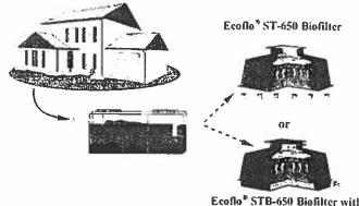
Ecoflo® STB-650 Biofilter with Submersible Collecting Bottom
