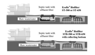
Your complete **septic treatment system** includes a septic tank with an effluent filter, one or more **Ecoflo<sup>®</sup> Biofilters** and, depending on the type of installation, a pumping station and/or a flow divider and/or a tertiary treatment system.
