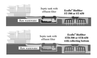
Your complete **wastewater treatment system** includes a septic tank with an effluent filter, one or more **Ecoflo**<sup>®</sup> **Biofilters** and, depending on the type of installation, a pumping station and/or a flow divider.
