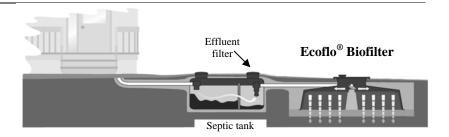
Your complete **wastewater system** includes a septic tank with effluent filter, one or more **Ecoflo**<sup>®</sup> **Biofilters** and, depending on the type of installation, an effluent filter, a pumping station, a flow divider.
