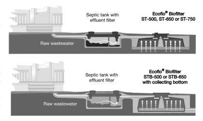
Your complete **septic system** includes a septic tank with an effluent filter, one or more **Ecoflo® Biofilters** and, depending on the type of installation, a pumping station and/or a flow divider.
