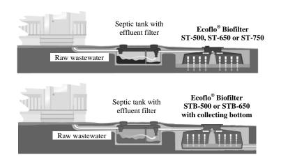
Your complete **septic system** includes a septic tank with an effluent filter, one or more **Ecoflo<sup>®</sup> Biofilters** and, depending on the type of installation, a pumping station and/or a flow divider.
