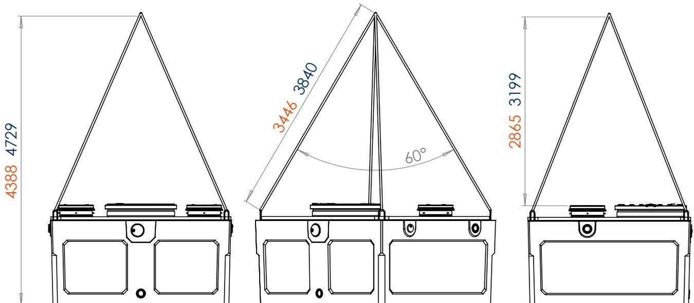
Levage EPARCO Compact Béton monolithe 5 EH
