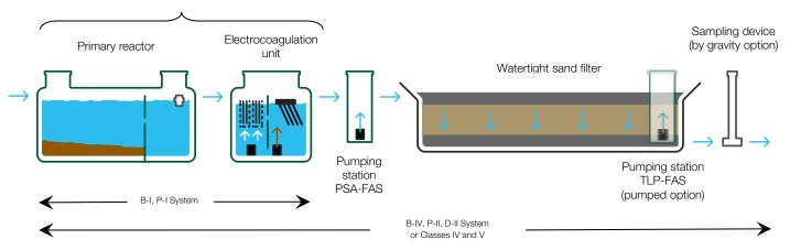
Phosphorus removal unit (DpEC) + Watertight sand filter
