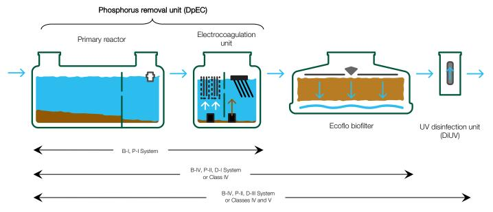
Phosphorus removal unit (DpEC) + Ecoflo biofilter + UV disinfection unit (DiUV)
