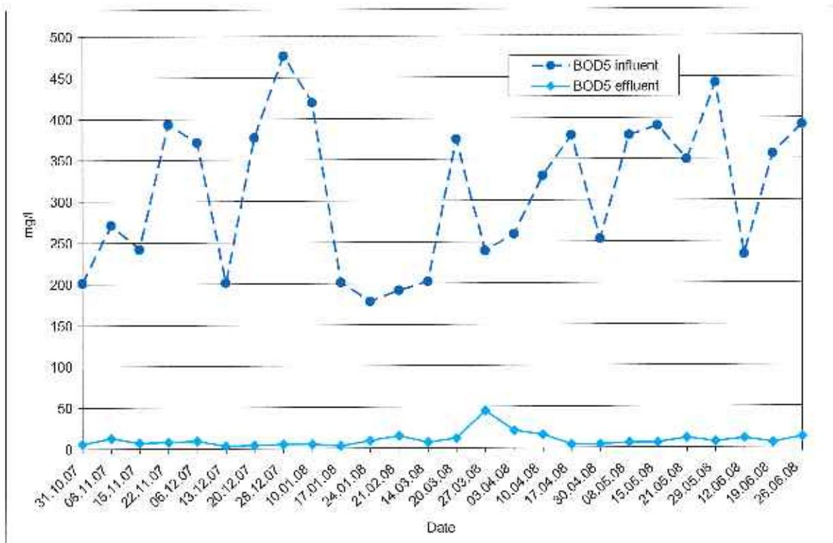
Figure 8: BOD<sub>5</sub> influent and effluent concentrations
