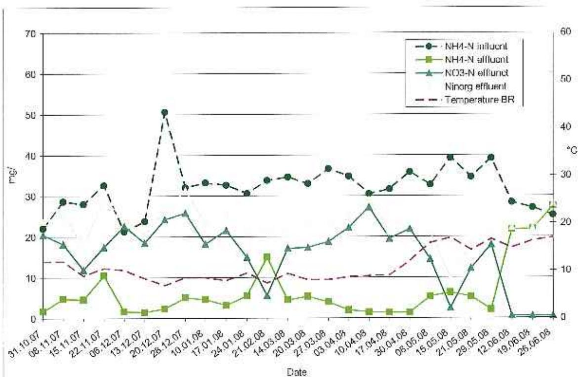
Figure 10: NH<sub>4</sub>-N influent concentration and NH<sub>4</sub>-N, NO<sub>3</sub>-N and N<sub>inorg</sub> effluent concentration
