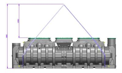
☐ Use webbed slings positioned around the tank for approximately every 1.8m of tank length. (2.5m diameter tanks). For 3.0m diameter tanks position every 2.0m. Ask Premier Tech for details. (Do NOT use any other item such as rope or chain)
