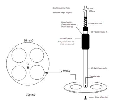
Probe fitted in PVC pipe pre-fitted to correct level in separator.
