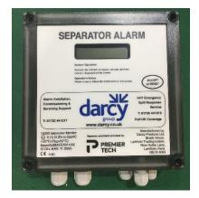
The standard system is supplied complete with an intrinsically safe control unit together with a high oil probe. The control unit is capable of monitoring up to 3 probe units, displaying their current status via a 2 x 16 display.
