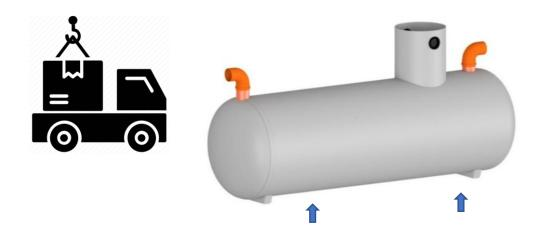
$\Box$  Use <u>at least</u> 2 x webbed slings positioned under the tank. (Do NOT use any other item such as rope or chain)
