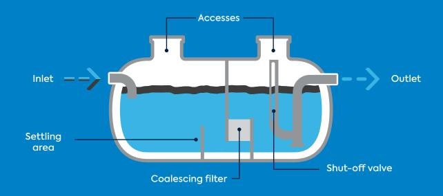
Hydrocarbon separators must be installed prior to any storage of rainwater from contaminated surfaces.
