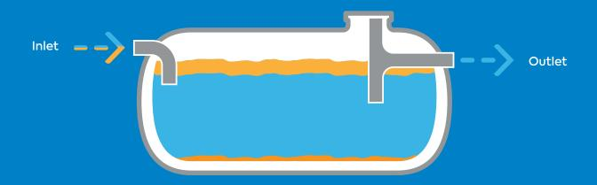
We recommend the installation of grease separators in conjunction with wastewater treatment systems.
