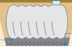
Lateral backfilling Stabilised sand - 100 kg oper m<sup>3</sup> of sand (3-6 mm). Backfilling well compacted. Width >200 mm. If the soil is clayey or difficult, the proportion is 200 kg of cement per m³ of sand
